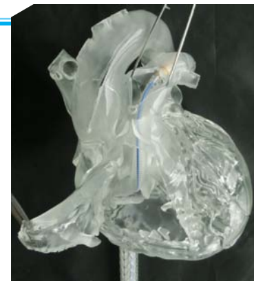
Fig.: Positioning of PERKAT in a silicon heart model: stent body lying in vena cava, outlet trunk bypasses right atrium and ventricle, while pigtail tip is in the pulmonary trunk.
