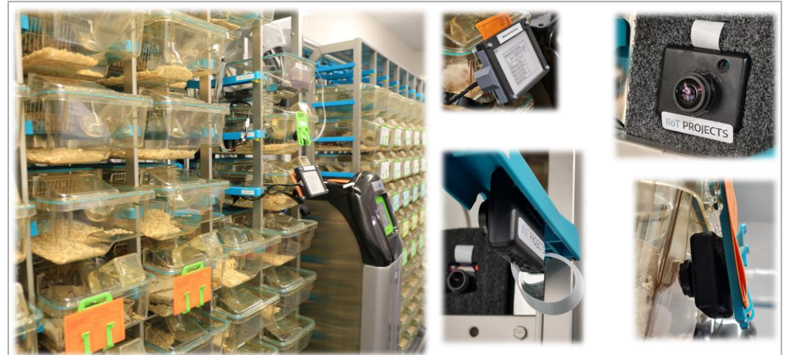
DIGI FRAME Retrofit system based on Techniplast IVC Emerald Line Home Cage 4 Cameras implemented and online VPN Secure access
