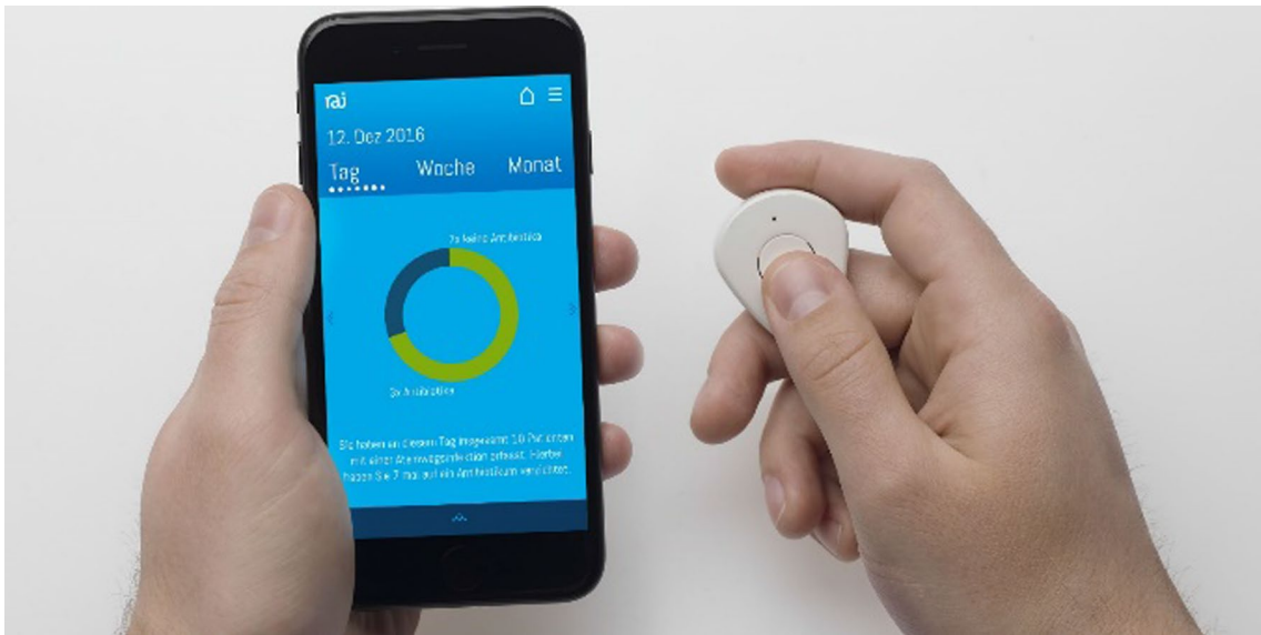
Fig. 1 GP self-monitoring App. The user clicks the button (right) for every ARI-patient with (blue) or without (green) antibiotic treatment
