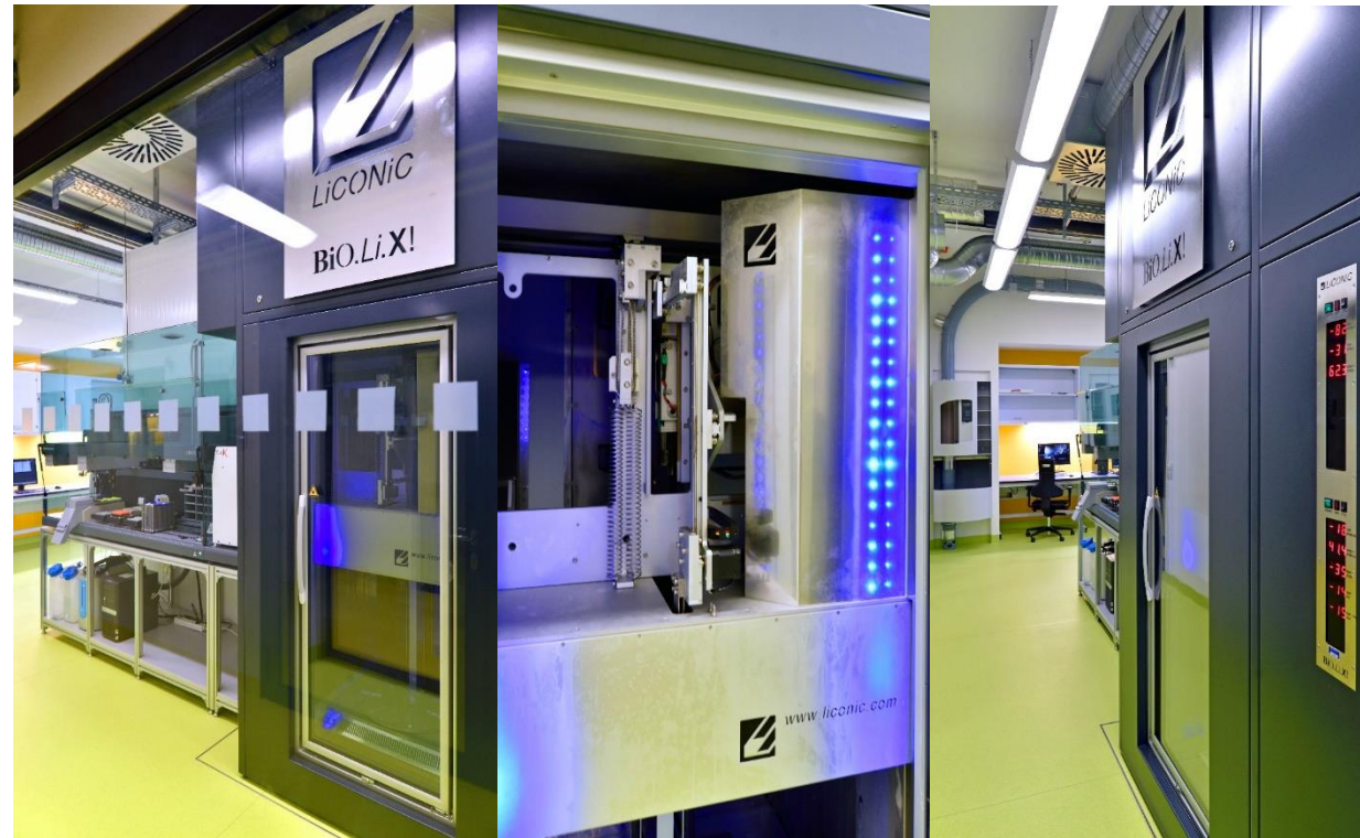
IBBJ 2.0: Automated -80°C Storage for 1.5 Mio tubes
