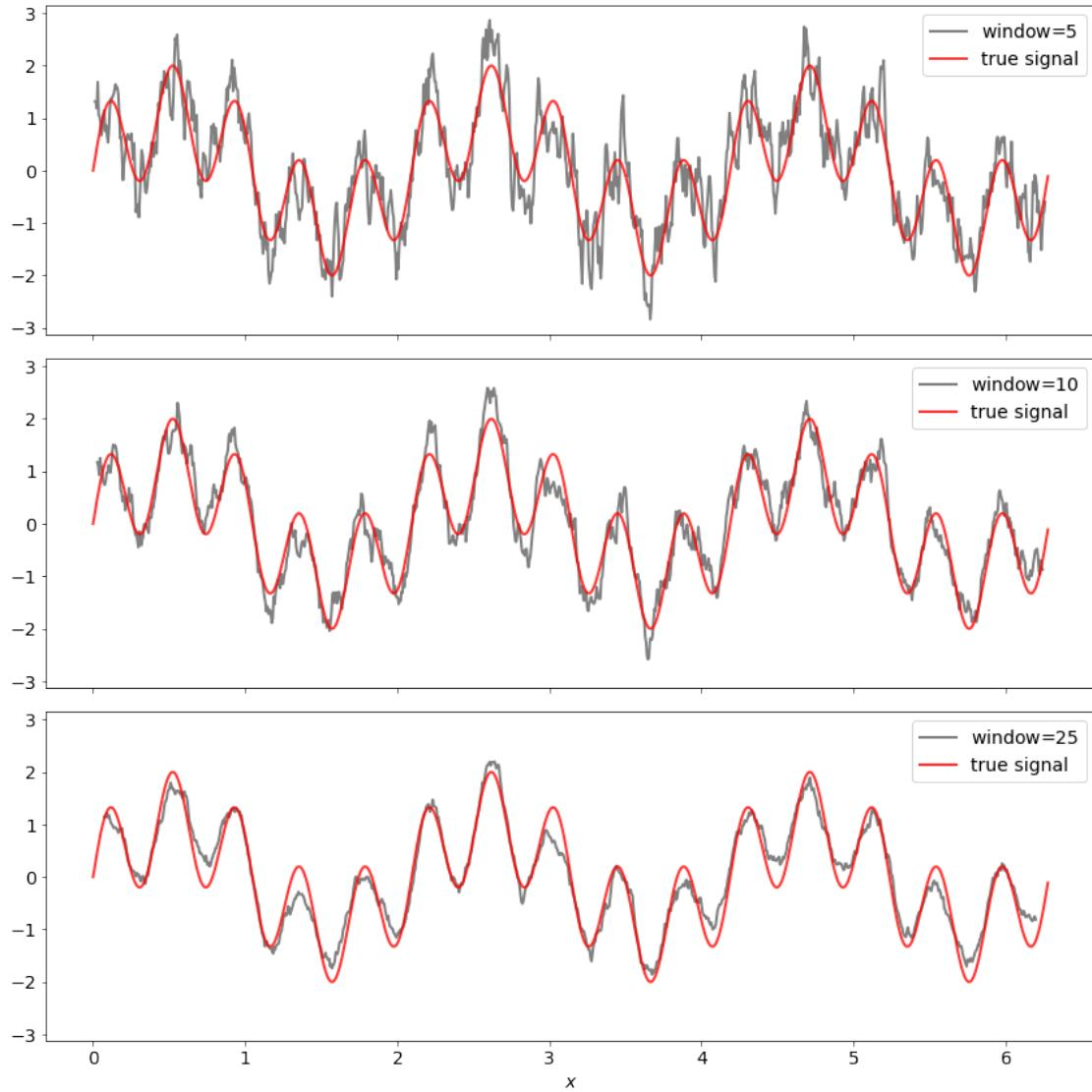
The sliding average can be interpreted as a convolution with a rectangular pulse of size  $w$  (where  $w$  is the window used in the averaging):
