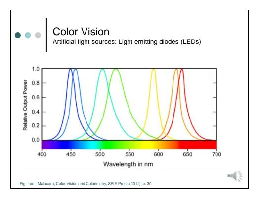
The same applies for light emitting diodes (LEDs). A light-emitting diode consists of several layers of semiconducting materials. Electrical voltage drives electrons from the n-layer and holes from the p-layer to the active layer, where they recombine and emit light. The light's wavelength depends entirely on the semiconducting material used.
