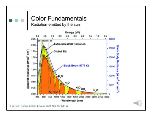
The radiation emitted by the sun (yellow curve) closely matches that of a black-body radiator at an effective temperature of ~5800 K.
